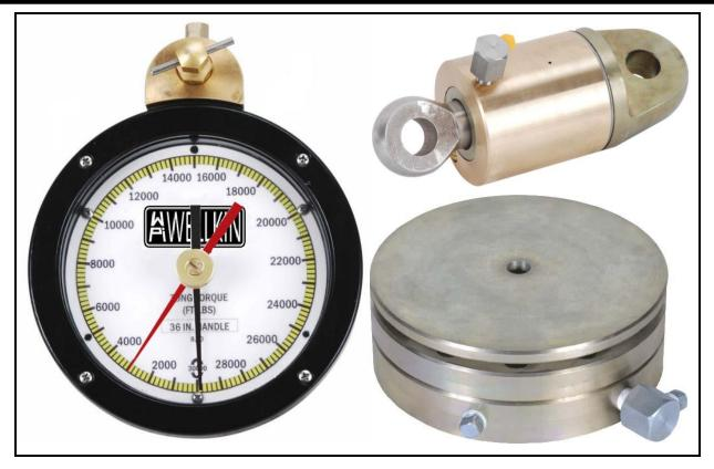
**Description:** The tong line pull and torque indicating system is used during the make-up of tubulars to get a reading of the applied load. Tong line pull gauges display in pounds, decanewtons, or kilograms, which can be easily converted to torque by multiplying by the handle or lever length. Tong torque gauges factor in the lever length so the gauge displays a torque value.
