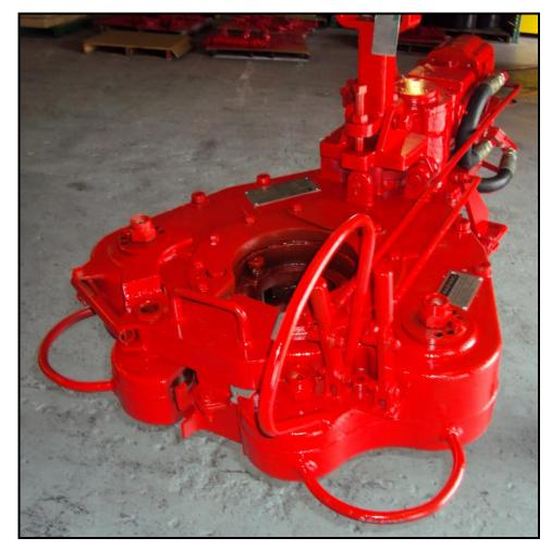
**Description:** The RS and RS-HT (High Torque) powered tubing tongs are an open face design. Tongs come complete with spring hanger and are less jaws/bushings and backup. The hydraulic power requirements are 2000 PSI at 35 GPM, and the tong has a 39" torque arm.
