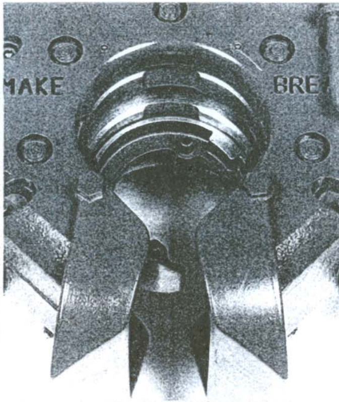
FIGURE 6 Tong out of time, brake drum not aligned
