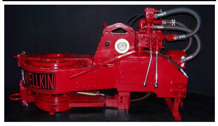
**Description:** The Model 58-93R hydraulic powered tubing tong is a closed head design. The hydraulic power requirements are 2000 PSI at 33 GPM, and the tong has a 36" torque arm.
