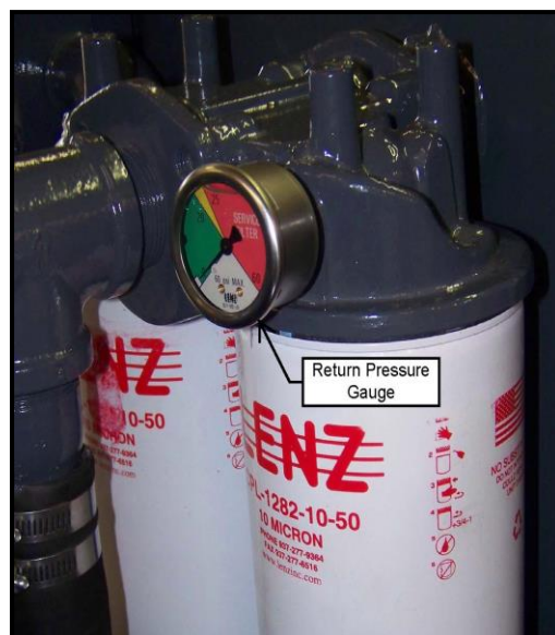
Figure 8: Return Pressure Gauge
