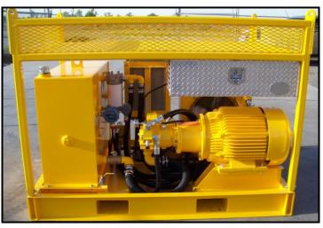
**Description:** Skid mounted, electric hydraulic power unit, for operation of close centered equipment such as drill pipe tongs or drill pipe roughnecks
