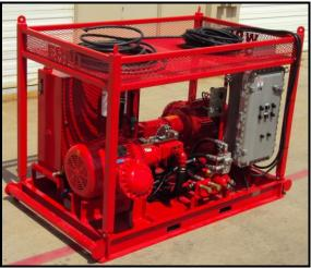
**Description:** Skid mounted, electric hydraulic power unit, for operation of casing and tubing tongs
