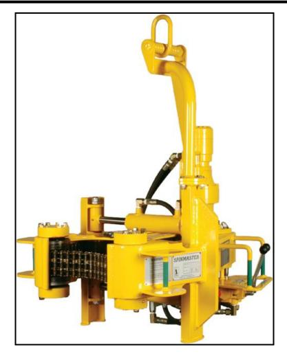
**Description:** The SPINMASTER drill pipe spinner is a roller chain design and is available in hydraulic or air operation. The hydraulic power requirements are 2000 PSI at 20 GPM. Air requirements are 240 CFM at 100 PSI. The compact design of the unit is easy to handle on rig floors. Changing the tool for different sizes is simple as only two pins have to be removed and then the drive assembly can be moved to the appropriate hole location.
