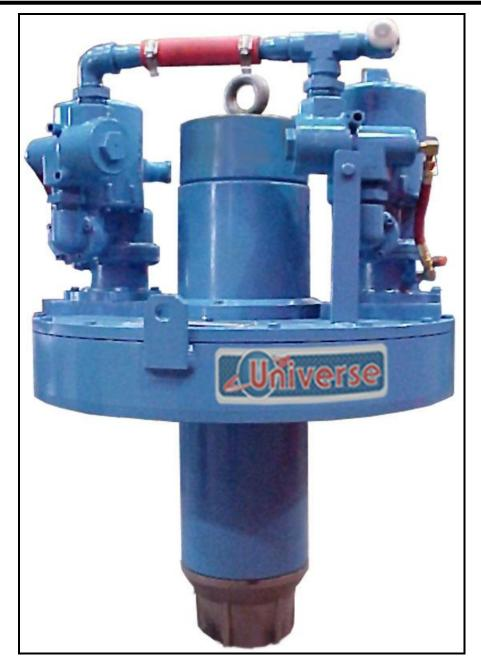
**Description:** Pneumatic kelly spinner, pin type, includes two non-lube air motors for CW and CCW rotation, with one 1" NPTF airline hookup and two 1/4" NPTF pilot line hookups, three turnbuckles, two 72 ft. x 1/4" pilot lines, one 72 ft. x 1" main airline, one 1-1/2" air filter, one 2-way/3 position hand operated control valve
